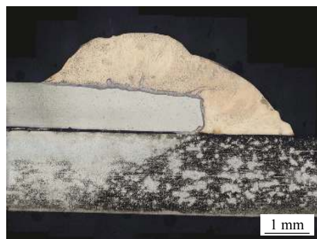
图3 TC4钛合金/镀锌钢旁路分流电弧钎焊接头形貌 Fig. 3 Cross-section of TC4/galvanized steel bypass-current arc brazing
